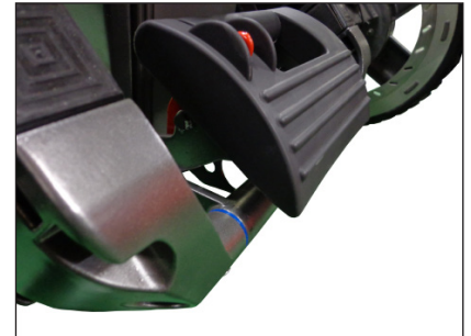
Not Locked Properly
